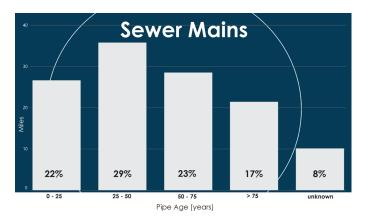
**Description**: The wastewater collection system consists of more than 120 miles of pipe. Many of the older pipes are 50 to 100 years old, undersized and at the end of their design life. Pipes are replaced programmatically as part of sewer-specific capital projects, roadway reconstruction and prior to annual paving. This project will fund the purchase of pipes and associated materials used to replace those pipes.
